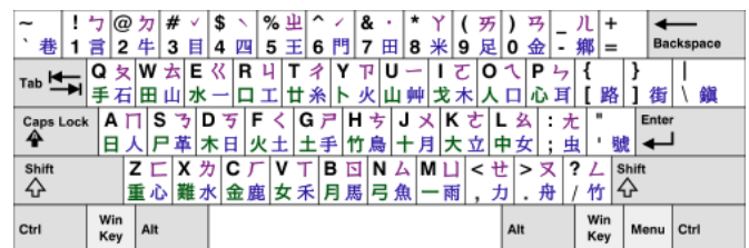
Chinese (Taiwan) keyboard layout, a US keyboard with Zhuyin , Cangjie , and Dayi key labels
